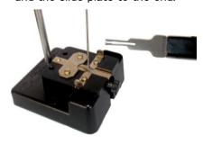
If it does not work properly, make sure if the wire follow the slide plate or Ering's position.
