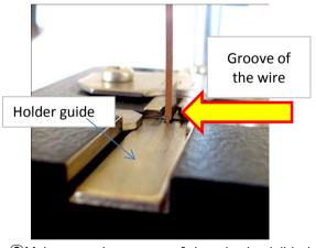
⑥Make sure the groove of the wire is visible in alignment with the holder guide.
